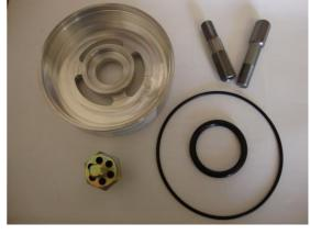
Remove the original filter bowl and its sealing ring (which may be stuck in the filter head). Fit the large diameter o-ring supplied into the groove in the filter head.
